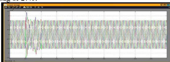
Fig 10. Simulation waveform for voltage sag mitigated using PWM switched autotransformer
